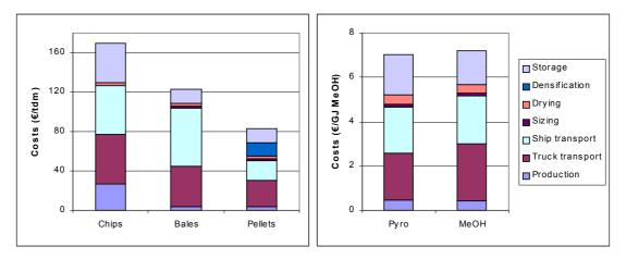
Figure 5.6: Chain costs for a Latin-American situation with an inland CGP in  $\ell/t_{dm}$  (woody biomass) or  $\ell/GJ_{fuel}$  (liquid fuels); international transport distance 10,000 km; conversion costs are excluded; ship transport only.
