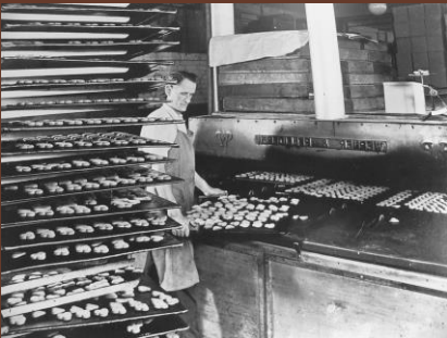
Biscuit production in the 18 metre long chain oven
